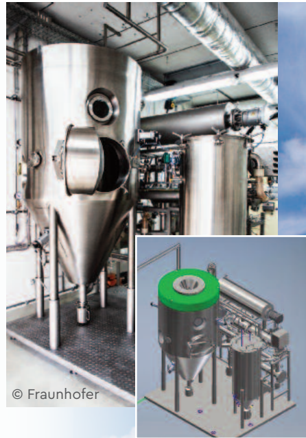
SPRAY DRYER EXPERO SDL-06 in a pilot plant for chemical products
