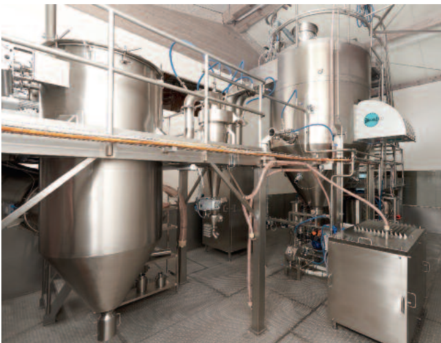
Pilot plant with homogenizer and safety equipment
