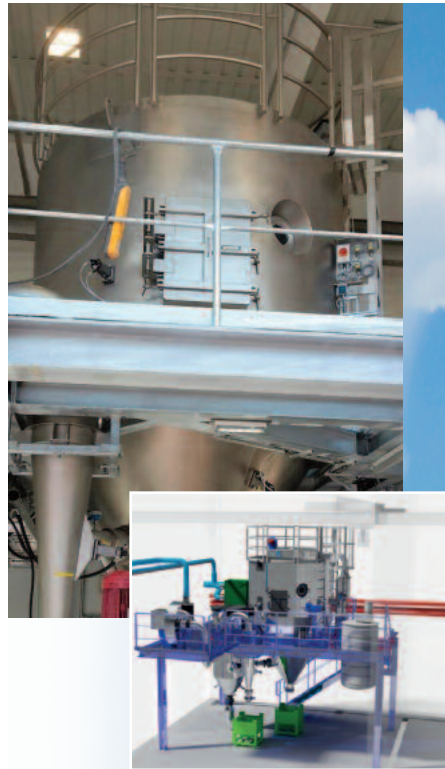
SPRAY DRYER INCUS RSD in the chemical industry for ceramic oxide/metal powder (inorganic pigments)
